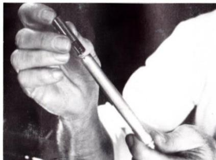
After cap is removed, insert 1.5 volts size AAA batteries as shown in photo (Fig. 5). Batteries are not supplied with this purchase
