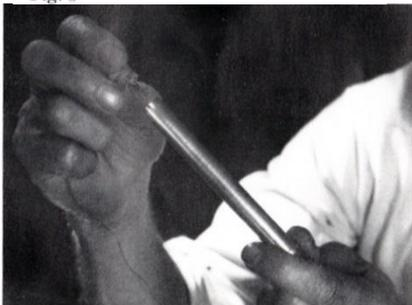
After battery pack is removed, remove cap (Fig. 4) as shown in photo by turning in counterclockwise motion.
