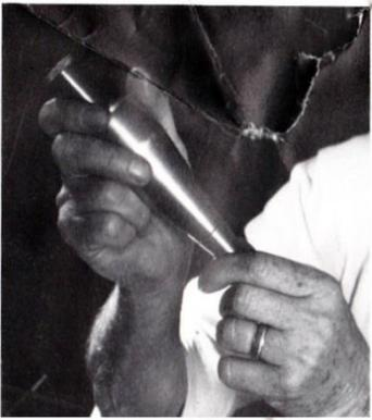
Hold body of plumb lite in either hand and turn barrel of plumb lite counterclockwise. (Figure 1)
