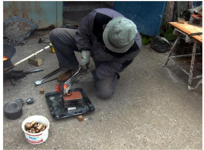
Brass + special chemicals heated to 1000 + degrees Celsius in a graphite crucible and poured into the mould.
