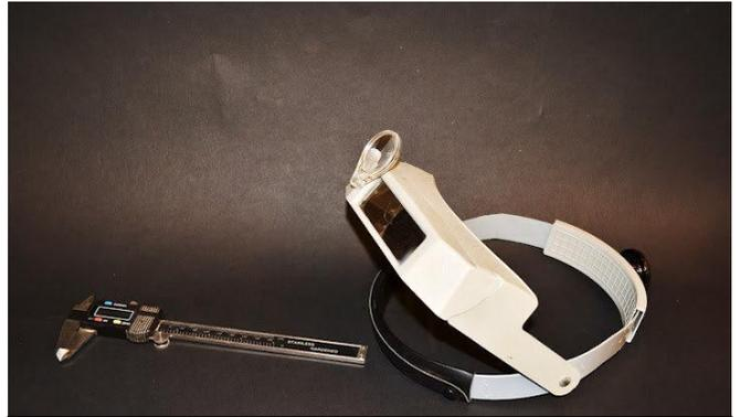
digital calipers and magnifier which are essential for doing this kind of work
