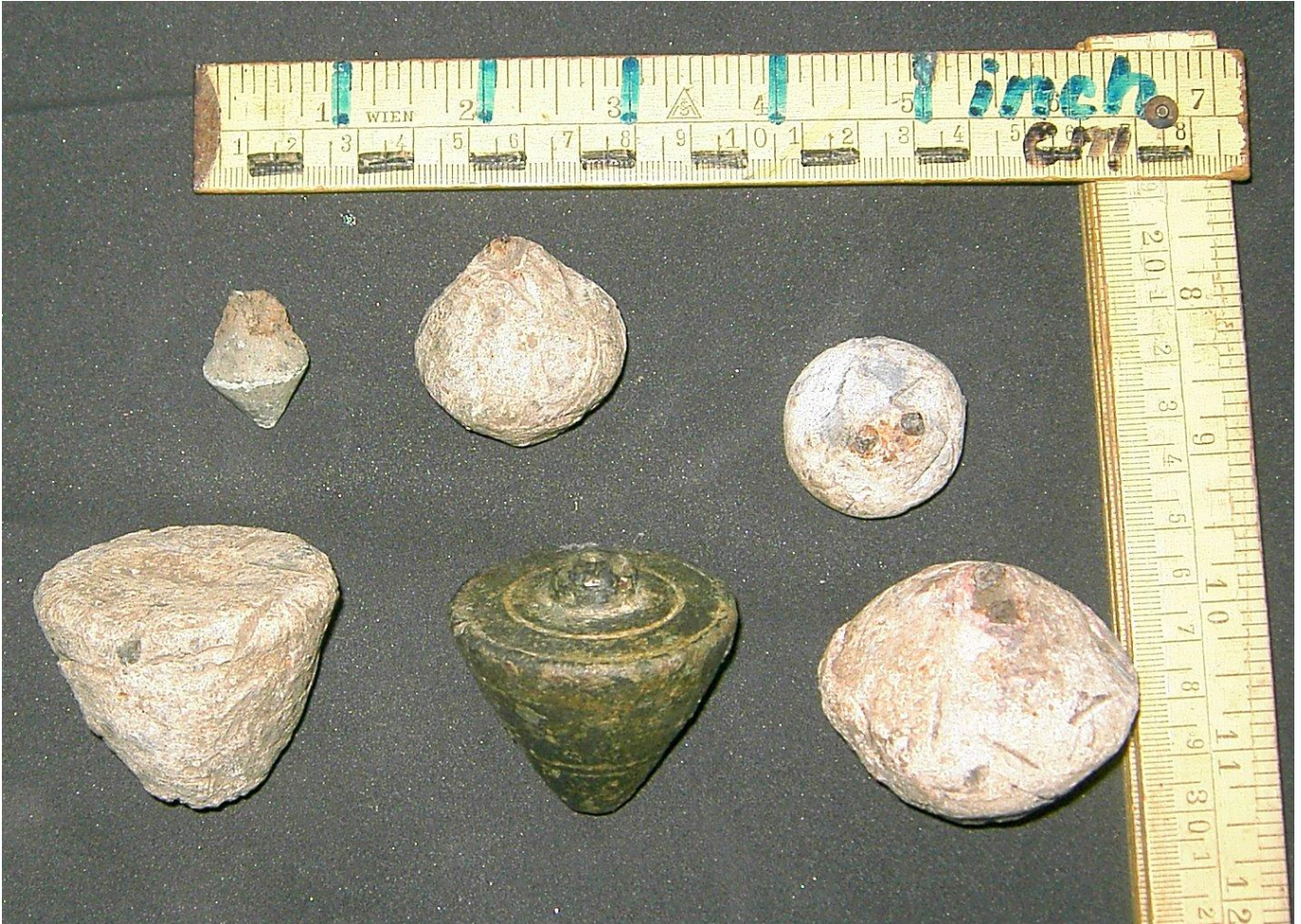
Collection Wolf Ruecker Roman plumb bobs of bronze 11oz and lead up to 21 oz.
