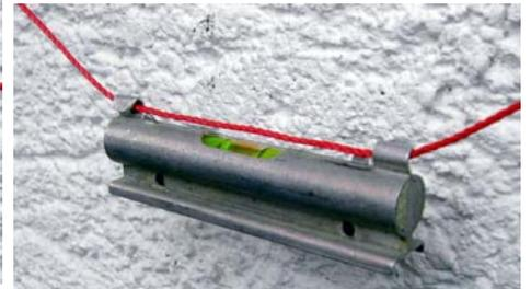
The MINING SURVEYORS used an inclinometer hanging on a STRETCHED line, to show the angle in the mines. See Wolf's PLUMB BOB NEWS 2009-03 MINING page 35
