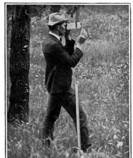
FIG. 65.—The mirror hypsometer in use.
