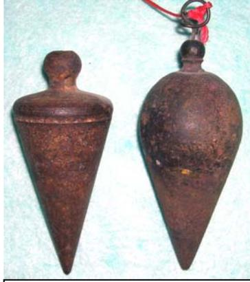
Fig. 23. Iron body with different shoulders
