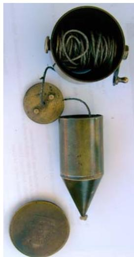
Fig. 44. Chalkline combination KUKA
