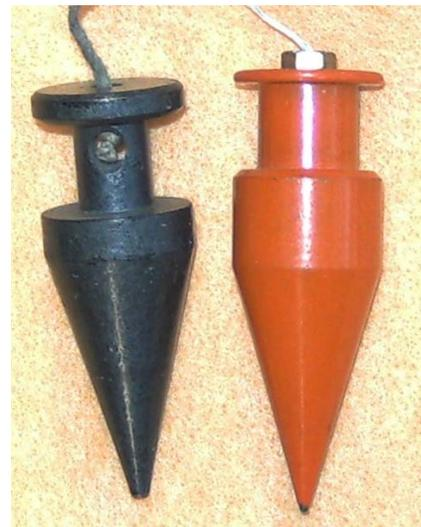
Fig. 36. Surveyors plumb bobs powder coated.
