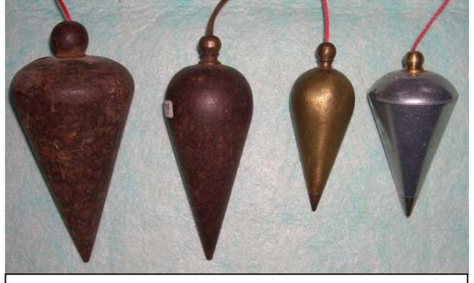
Fig. 24. Germany Iron, iron round shoulder, brass and zinc die cast
