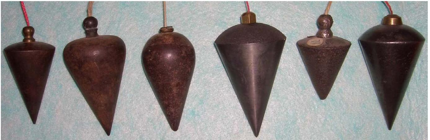
Fig. 25. Germany: Different shapes / shoulders of iron and cast iron (turned) plumb bobs
