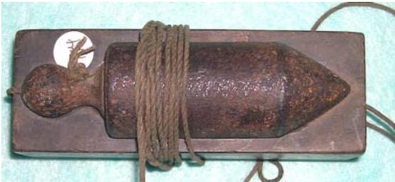
Fig. 26. Masons p b with adapted wooden spacer.
