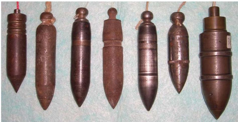
Fig. 37. Plumb bobs built from munitions.
