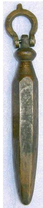
The body of these plumb bobs was of one material only. At that time they did not have a hardened steel tip by another material or a combination of different materials. Unfortunately we don't have pictures that show the production of plumb bobs in that time ☹.
