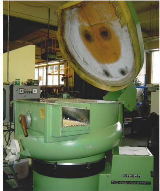
machine for cleaning and polishing
