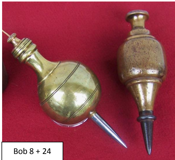
FIG. 135. TYPE OF PLUMB-BOB USED IN PLUMBING MERIDIAN DOWN A SHAFT.
