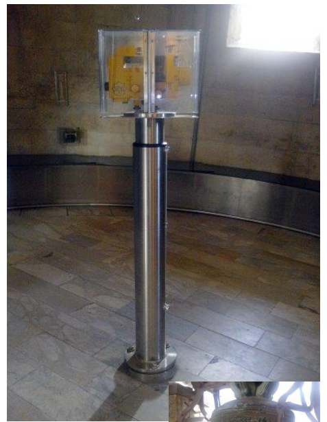
Fig. above: The installation inside the bell tower to verify the data of the LEANING bell TOWER Fig. left: Surveyors at work in front of the tower
