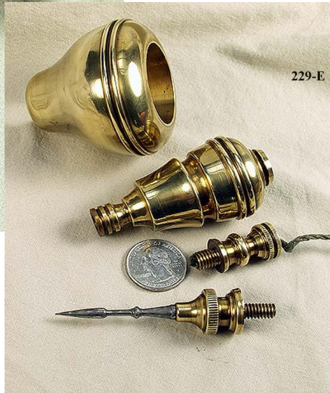
# 229. Spectacular, crisply detailed, plumb bob within plumb bob. Unscrew the ornate steel tip and remove the main body, which houses an equally, but smaller, ornate plumb bob. Exquisite craftsmanship and design.
