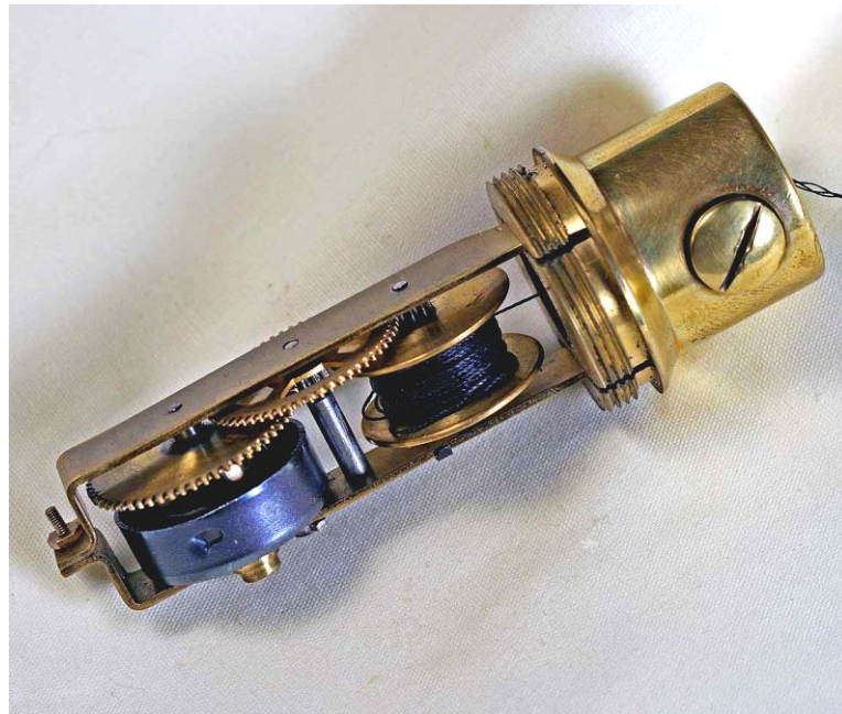
# 481. Rare hexagonal w/ "clockworks" internal winding mechanism and key. KNAUS patent 3,027,977 – 1962
