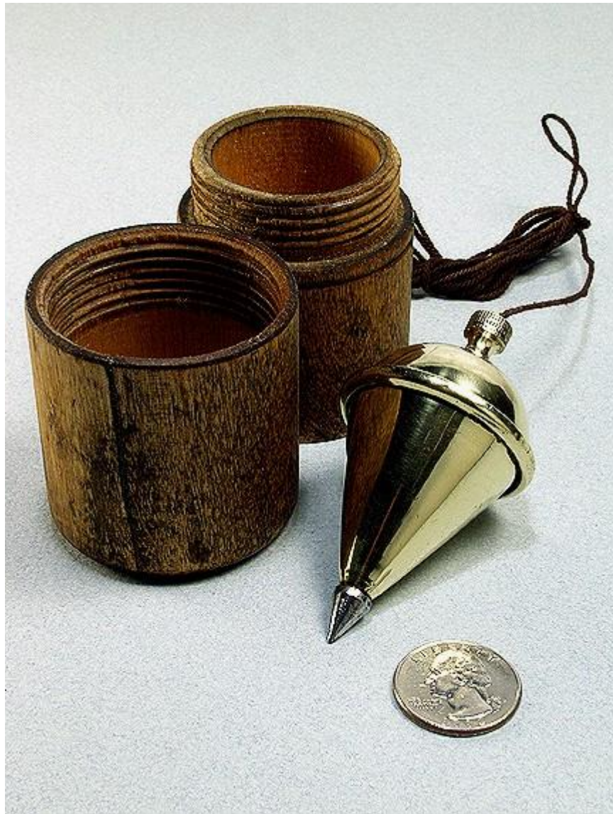
# 208. PERFECTION plumb bob, patented, April 25, 1905, 3-1/8", 12-7/8 oz. Purchased in snug fitting simple turned wood case. Crack in case does not spoil thread function. Decorative "dado turning" below joint of top and bottom halves. Made by TOWER & LYON, NEW YORK
