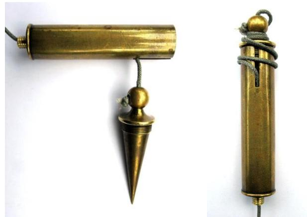
*a small, one piece, solid brass construction that screws into a brass tube for protection - everything normal to this point. Furthermore, the tube has a slit at the open end which allows the exit of the line, but this is impractical, because the line is twisted and tangled when the plumb bob is screwed into place. There is also a threaded opening at the closed end of the tube, with something possibly missing.*
