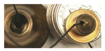
THROUGH......TIGHTENING THE CAP SIMPLY CLAMPS THE STRING BETWEEN THE CAP AND THE BODY.....THUS, NO MORE MINISCULE PART TO LOSE
